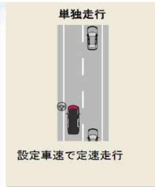
Running alone Run in a constant speed at the set vehicle speed
