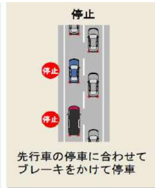
Stop In accordance with the stopping of preceding car, brake is applied and stopped.
